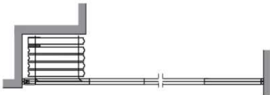
Two Point Suspension & parallel to track
